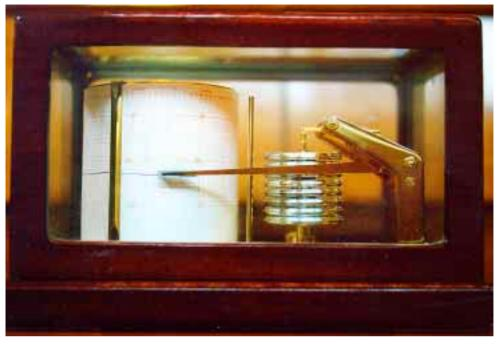
A Weems & Plath recording barometer. This unit runs on a single AA battery that lasts about six months. The paper chart takes a week to go around the drum. Having a visible trace of what the barometric pressure is doing makes it a lot easier to get a handle on the coming conditions.
