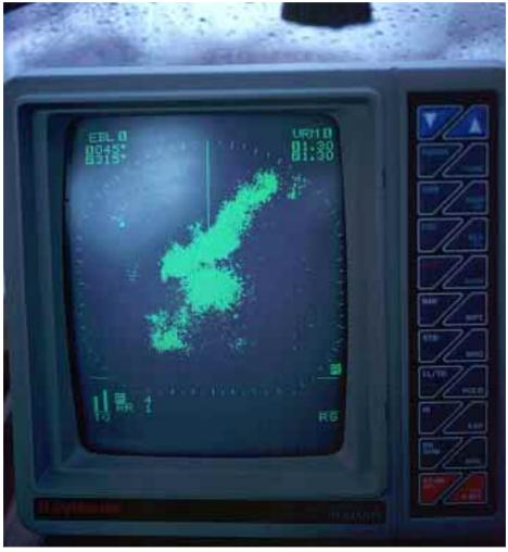
An early model Raytheon 41X radar with enclosed radome. This photo was taken coming up through the tropics in a moderate squall (you can see here about six miles in length). About 25 knots of breeze and strong rain occurred for about 20 minutes.
