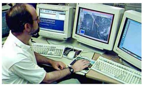
Joe Sienkiewicz, lead Marine Forecaster, working on the morning Pacific regional chart and text package. Forecast text is shown on the left screen and a satellite image on the center with model output overlaid. On the right screen is model output data. These monitors are tied to the central computer server and can call up any of the data or images on any of the screens.
