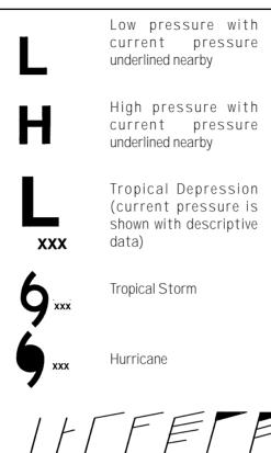
Wind feathers indicate the strength (in knots) and direction of the wind. The head of the arrow (without feathers) points in the wind direction. A single small barb is five knots. A single long barb is ten knots. A flag is 50 knots (the feather to the right is for 65 knots). When the head of the feather has a circle this indicates the report is from a ship or buoy.
